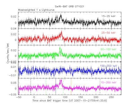
Fig.1: BAT Lightcurve. The light curve is in the 4 individual plus total energy bands. The black and green dotted lines show the time interval of T90 and T50 respectively. The blue solid line is the spacecraft slew start time and the orange solid line is the spacecraft slew settled time.
